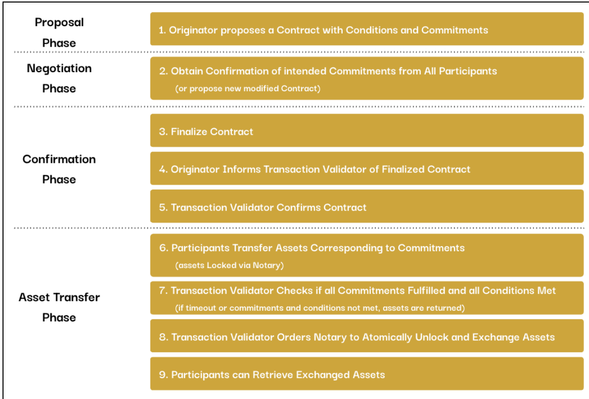
Sample Contract-Based Transaction Execution Flow
